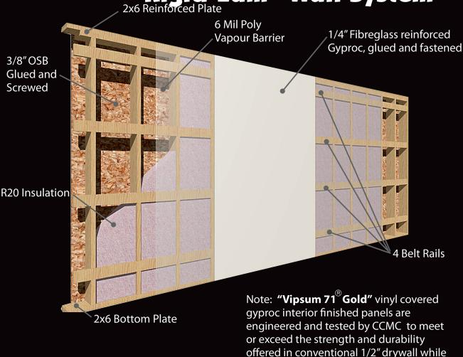
Regent Homes now offers the new and improved Rigid-Lam wall structure on all of their housing products. This unique system further improves the overall strength of the home making it the most superior structure in the industry today. A strong wall means better transportation, improved longevity and better resale value.
